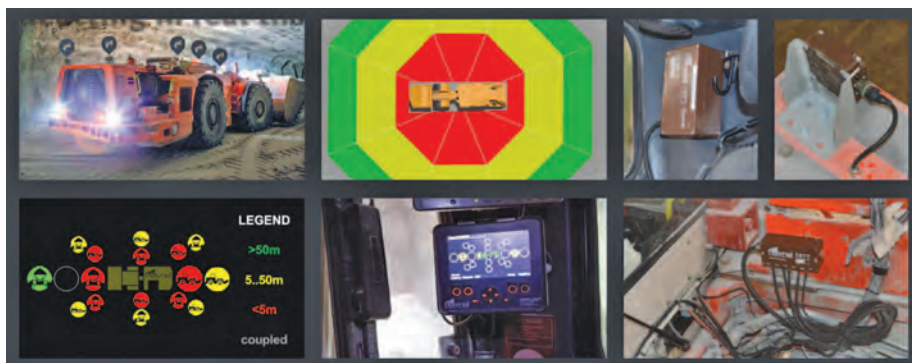
The iProximity 5G system being developed by indurad includes both radio and radar sensors to provide a highly accurate solution
