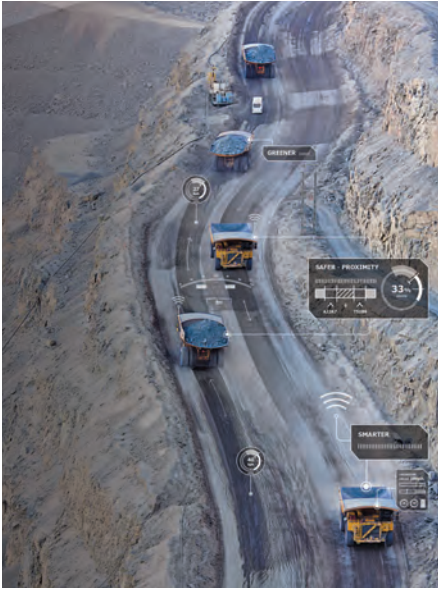
The new Generation 3 CAS from Wabtec can curve proximity detection beams
